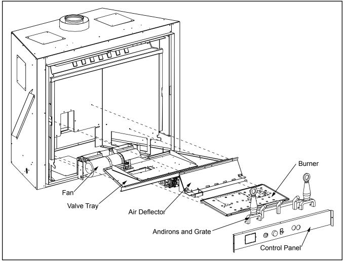
Figure 45: Removal of DV42DX Burner and Fan.
